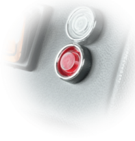
FILTER CLOGGING INDICATOR Filter clogged or need to be replaced indicator light
