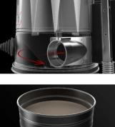
The tangential inlet facilitates the cyclonic effect to deposit the collected material in the container. Filtration is ensured by a polyester star filter in class M (filtering efficiency 1 micron) with high filtering surface area, which guarantees air passage even with a dirty filter.
