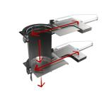
DOUBLE DISCHARGE WITH ELECTRO-PNEUMATIC DAMPERS System with dampers that open alternately to allow the material to be discharged and the vacuum to be maintained at the same time.
