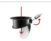
DISCHARGE WITH COUNTERBALANCED FLAP The material is automatically discharged every time suction is stopped.
