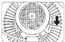
Check that the direction of rotation of the pump matches the one indicated by the arrow in the figure.
