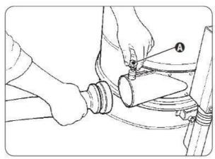
Insert the appropriate accessory for the type of vacuuming from the opposite side of the hose
