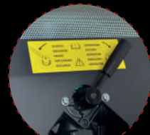
Reverse Flow Discharge system
