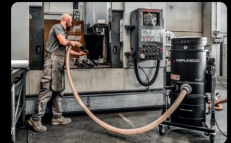
Metal chips cleaning from a CNC machine
