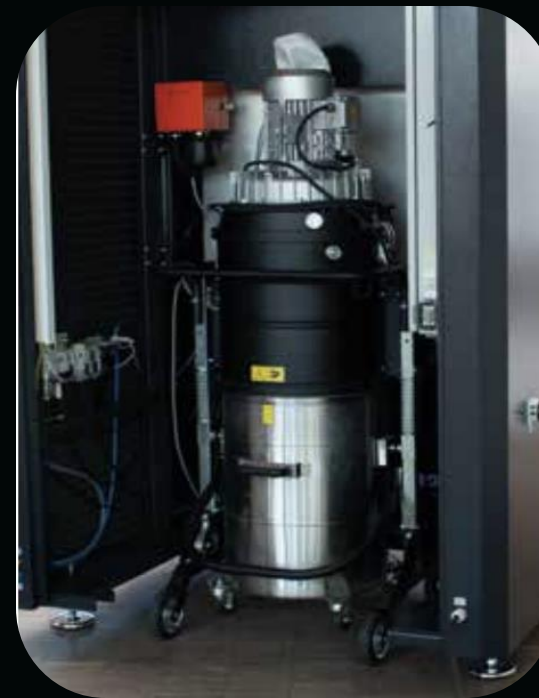
Industrial vacuum integrated into the depowdering station
